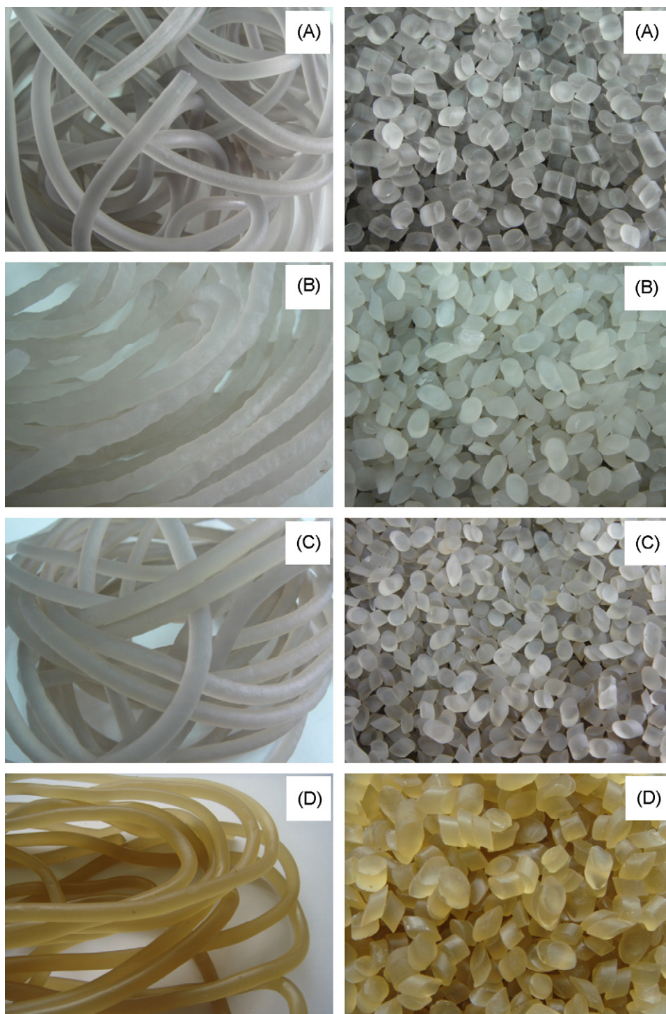
Fig. 1. Appearances of different TPS extrudates (left) and pellets (right): (A) TPSN, (B) TPSTW, (C) TPSLA and (D) TPSZE.
